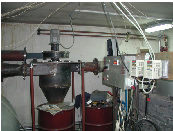
Fig. 3. The cyclone-type particle precipitator
